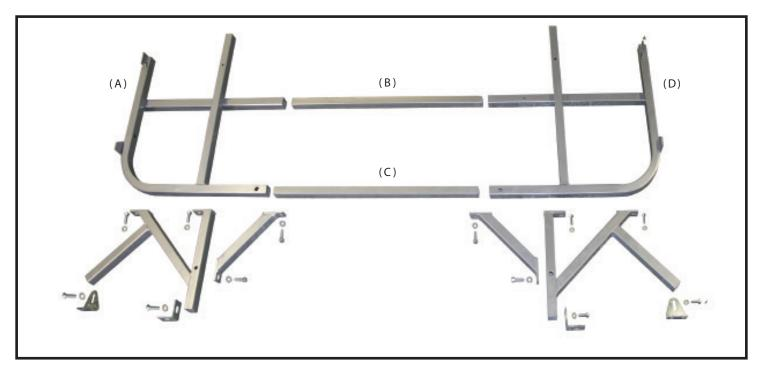
2. Using the bolts and washers supplied, bolt the above items together and then add the floor mounting brackets as shown below.
