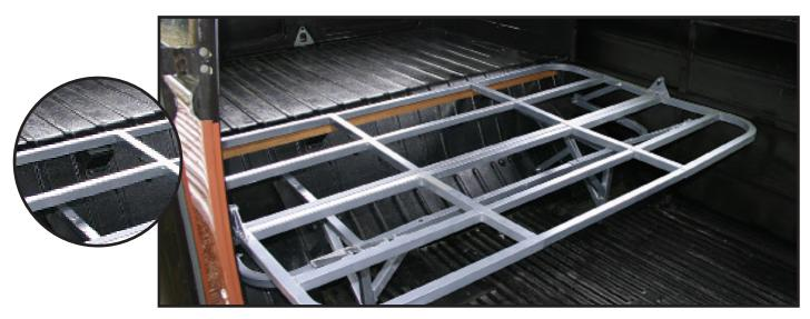
9. Cut a thin sheet of wood or MDF to the correct shape and screw it over the frame, followed by foam and your choice of fabric. The base of the seat could also be 'boxed in' with wood or MDF making a useful storage area under the seat
