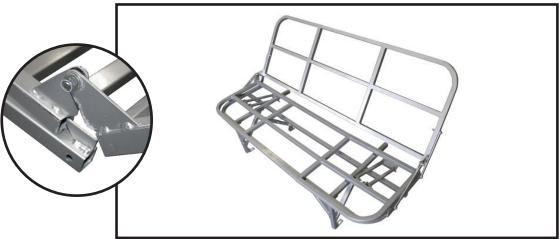
6. Place the frame in the van, making sure that it is level. Using the feet as guides, drill holes through the floor and rear bulkhead, then bolt the whole unit to the floor.
